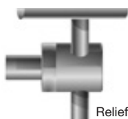
Backpressure valve on tee for pressure relief
